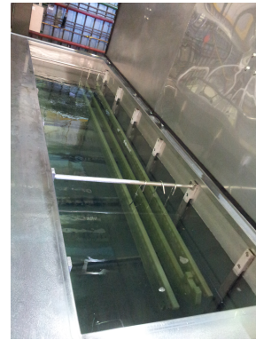
Figure 32: Sonic bath with two percent solution of Elma Clean 65.
