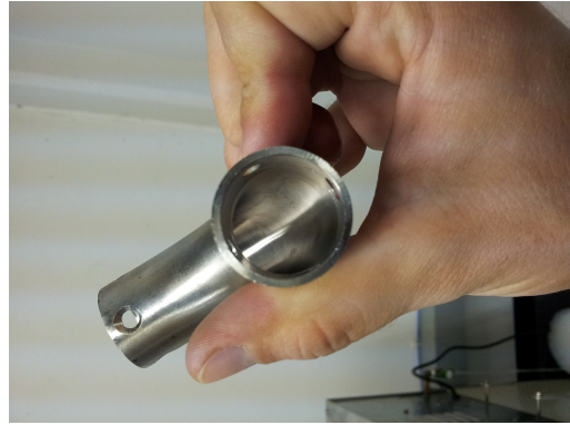
Figure 17: L-bow after manual removal of grease and dirt
