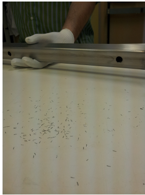
Figure 1: Small machining pieces inside welded suport beams.
