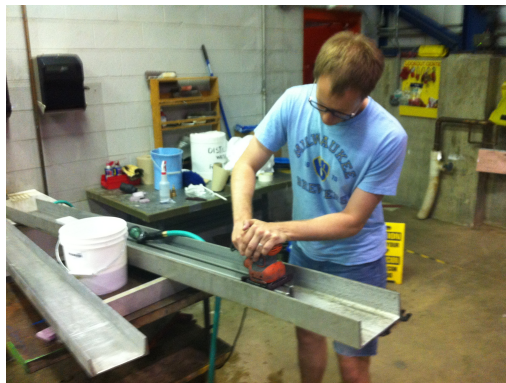
Figure 7: Sanding of the beams for very dirty parts.
