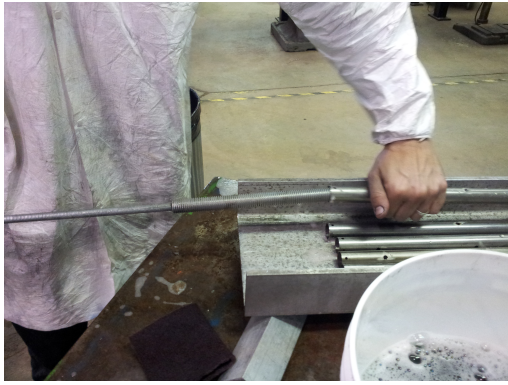
Figure 21: Reaming of the pipes.
