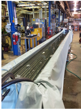
Figure 23: Soaking of the pipes.
