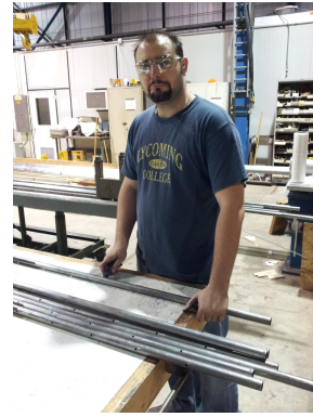
Figure 22: Deburring of the pipe holes.
