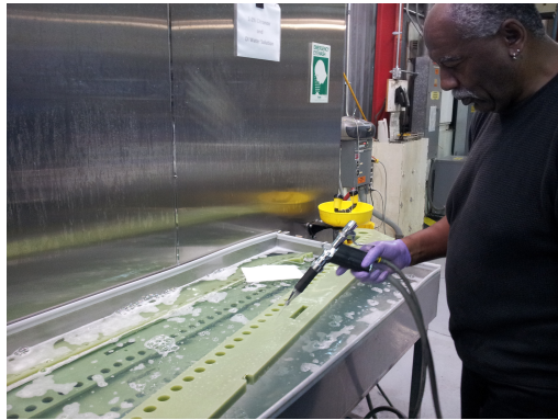
Figure 31: Rinsing after pre wash with a water jet.
