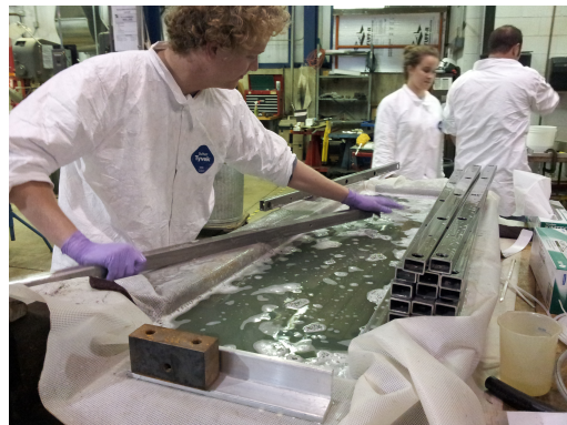
Figure 6: Soaking of beams in a simple green solution.
