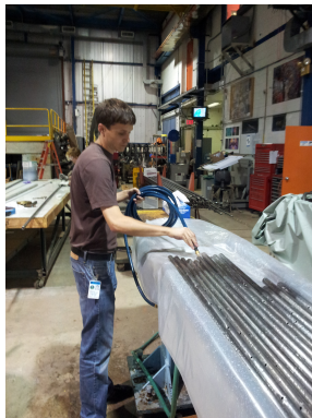
Figure 25: Rinse of the pipes.
