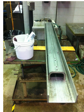
Figure 2: C channel used for rinsing and cleaning larger metall parts.
