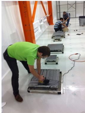
Figure 3: Preparation of the DAB TPC assembly tent Sanding of the supports.
