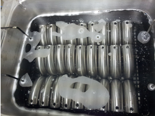
Figure 18: Ultrasonic bath with heated two percent Citronox solution.
