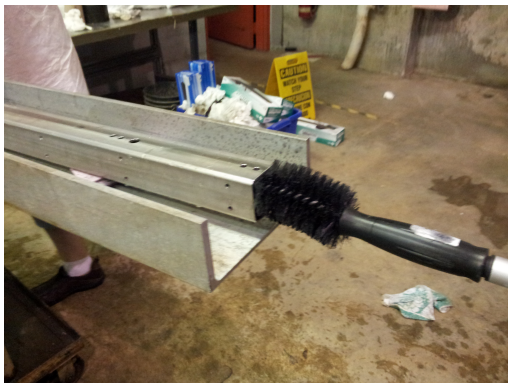
Figure 5: Cleaning of beams with a special brush.
