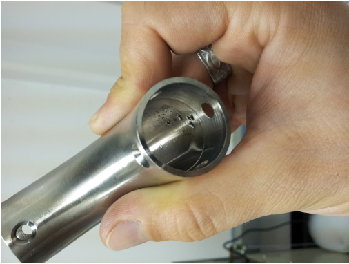
Figure 16: L-bow before manual removal of grease and dirt.
